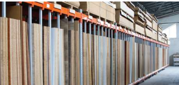
When stacking vertically, provide support and ensure that the gap between boards is uniform.
