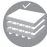
Minimum 4-5 battens should be provided at maximum spacing of 50 times of the thickness of the boards, but not exceeding 800 mm distance, center to center.
